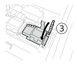
(12) Connect the flat cable to the carriage board.
