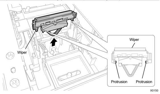
(9) Insert a new wiper into the printer from above.
