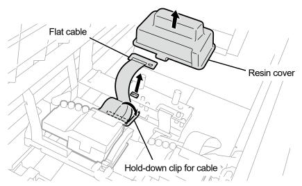
(10) Unlock the print head, and remove the print head.
