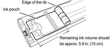
(7) Open the lid of the cartridge and place the ink pouch in its correct position.
