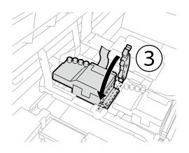
(20) Connect the flat cable to the carriage board.
