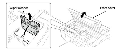
(7) Take out the wiper cleaner from its packing bag, and remove it from its protector.
