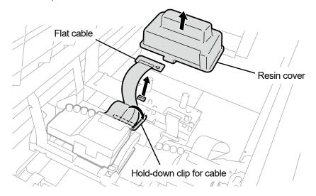
(17) Unlock the print head, and remove the print head.
