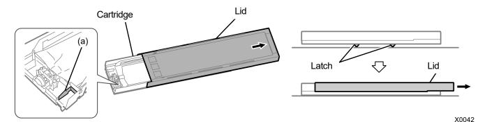
(5) Pinch the latch at the front end of ink pouch, and draw out the white ink pouch from the cartridge.
