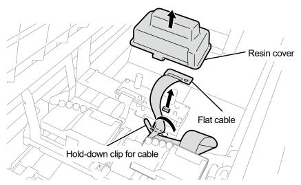
(9) Unlock the print head, and remove the print head.
