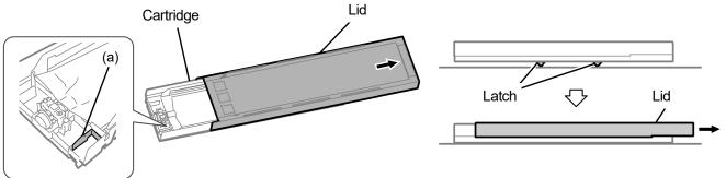
(5) Remove the maintenance solution pouch from the cartridge, and put the white ink pouch in place.
