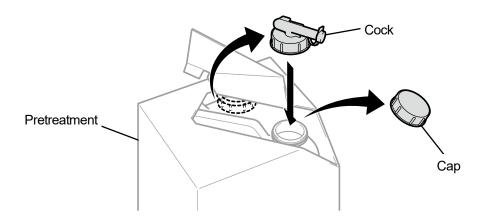
(3) Orient the pour spout of cock in the position as shown in the figure below.
