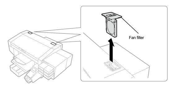
(5) Mount a new fan filter to the frame of filter case.
