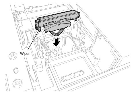
(10) Place the spring under the wiper on the maintenance unit latch.
