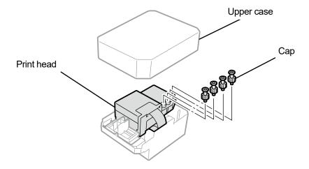
(14) Remove each tube from the print head to be replaced with a new one, then attach each of the new caps which are removed from a new print head to each tube, while exercising care to prevent any ink from being spilled.
