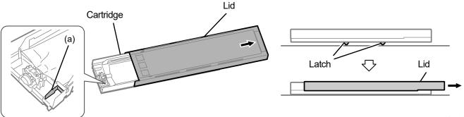
(5) Pinch the latch at the front end of the ink pouch, and draw out the white ink pouch from the cartridge.
