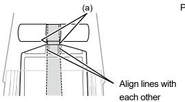
Place the pouch in a straight alignment with the cartridge
