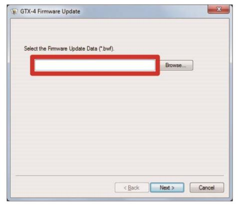
(4) Make a connection of the USB 2.0 cable or LAN cable between your PC and the printer, and update your firmware by performing the on-screen procedures.
