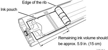
(3) Open the lid of the cartridge and place the ink pouch in its correct position.
