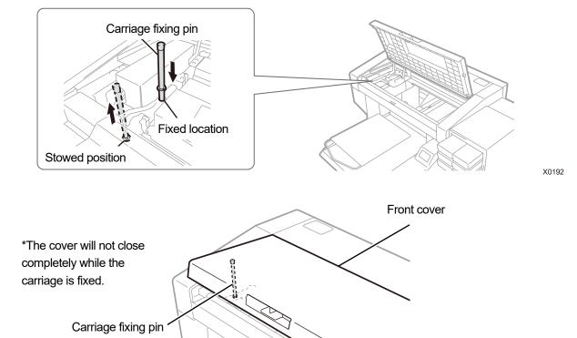
(3) When the current state is brought to an available condition to turn on the power, pull out the carriage fixing pin, return it to its stowed position and reactivate the printer.
