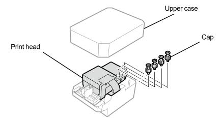
(6) Remove each tube from the print head to be replaced with a new one, then attach each of the new caps which are removed from a new print head to each tube, while exercising care to prevent any ink from being spilled.
