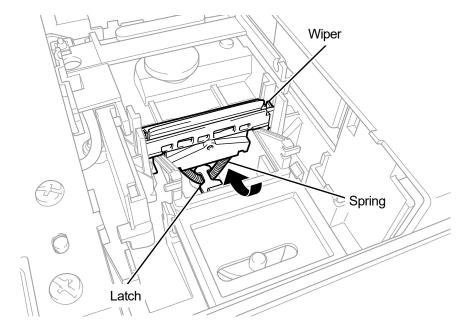
(8) Remove the wiper from the maintenance unit.
