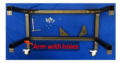
• Mount the entire front section on the stand by lining up the bolts with each of the support arms holes.
