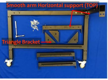
• Repeat the process from step one with on the opposite side top horizontal support and triangle bracket. When putting in the triangles it helps to tilt the support arm back slightly to get the triangle seated.
